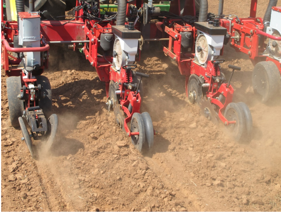
Figure 2. Closing systems on the AGCO planter. The left row shows the standard system while the two center rows have the alternative closing system.
