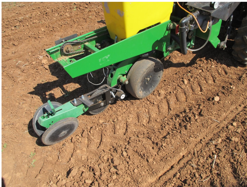
Figure 1. One row planter developed at OSU to orient and place corn seed.
