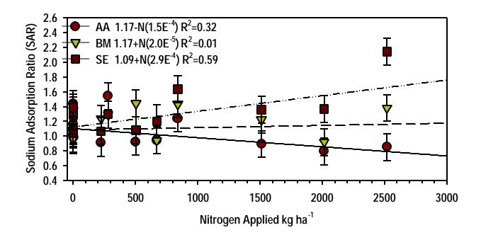
Figure 3 Sodium Adsorption Ratio (SAR) at the 0-15 cm depth as a function of cumulative annual applications of anhydrous ammonia (AA), beef manure (BM), and swine effluent (SE) in a continously cropped, convetionally tilled corn production system located at OPREC, Goodwell, OK. Data represents three years of cumulative applications.
